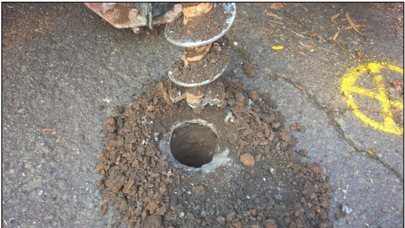
Photograph 2. Soil conditions (fill material) encountered (brown clayey loam with gravels and asphalt pieces) at BH15 from approximately 0.05-0.3 m BGL.
